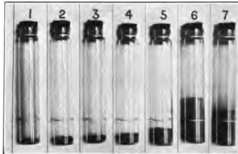
FIG. 2.—RELATIVE AMOUNTS OF DIFFERENT SIZED PARTICLES COMPOSING A LOAM SOIL.
